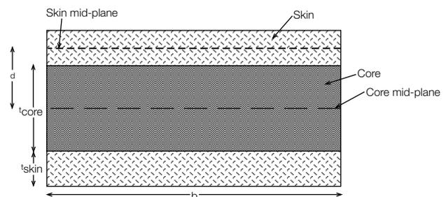
A sandwich's stiffness is proportional to the cube of the increased core and skin thickness
